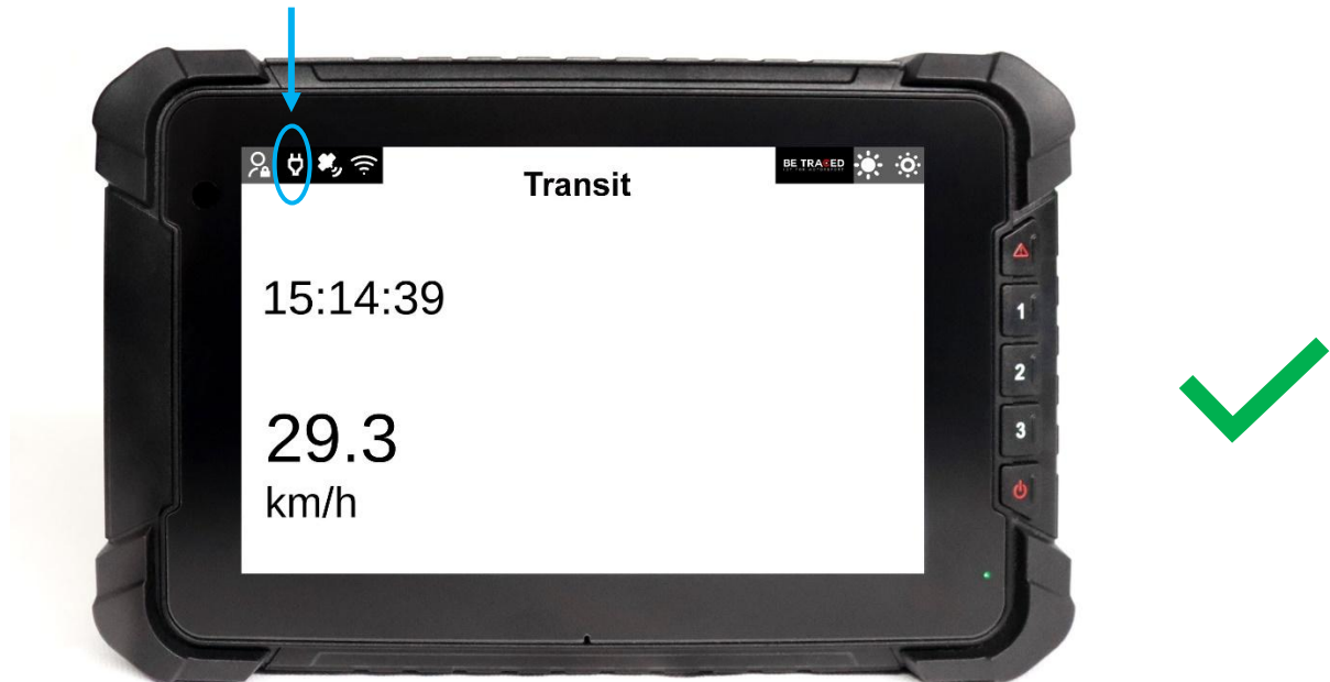
Figure 1 - White power light: device powered correctly
