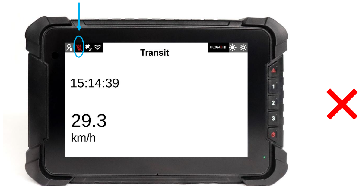
Figure 2 - Red power indicator light: device not powered
